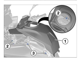
• Remove cover (1) to the top, detaching it from the retaining clips (2) and from the retaining lugs (3) on the left and right.
