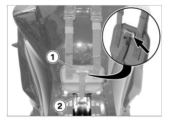
• Work strap from rear attachment element (1) through standard provided holder (2) and close closure (arrow).
