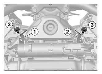
• Fit retaining plate on left (1) and right (2) and install bolts (3).
