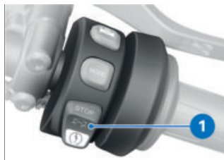
1 Emergency-off switch (kill switch)
