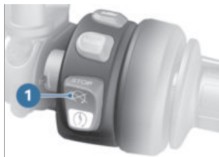
1 Emergency-off switch (kill switch)
