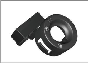
To verify the authorization of the ignition key, the electronic immobilizer exchanges information with the ignition key via the ring aerial.
