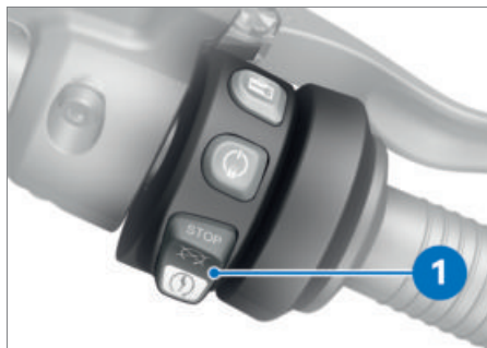
1 Emergency-off switch (kill switch)
