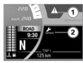
Warnings for which there are no separate warning lights are shown using the general warning light 1 in combination with a warning symbol such as 2 on the multifunction display. The 'general' warning light is yellow or red, depending on the urgency of the warning.
