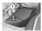
Unlock and lock the lock 1 of the storage compartment using the ignition key. • To open the lid, press the unlocked lock barrel down
