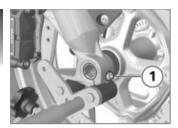
Tighten right axle clamping screw 1 to specified torque.
