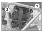
Begin by connecting one end of the red jump lead to the positive terminal 1 of the discharged battery and the other end to the positive terminal of the donor battery. If the 12 V battery is installed incorrectly, or if the terminals are exchanged (e.g. when jump-starting), this can result in the fuse for the alternator regulator blowing.◀
