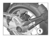
Conduct a visual inspection of the brake pad thickness. Viewing direction: between splash guard and rear wheel toward brake pads 1.
