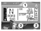
Warnings for which no separate warning lamp is provided are signaled by the general warning lamp 1 and are accompanied by a warning symbol in area 2 or by a warning notice in area 3. The universal warning lamp shows red or yellow, depending on the urgency of the warning.
