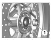
Mount spacing bushing 1 on left side in wheel hub.
