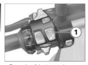
Press the 1 button and continue to hold it down until the status indicated by the ASC warning lamp changes.
