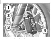
Detach wheel speed sensor lead from retaining clips 1 and 2.
