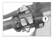
Press and hold button 1 until ABS warning lamp's display changes.
