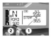
In the case of outside temperatures below 37 °F (3 °C), risk of ice formation exists. The display automatically switches from any other mode to outside temperature reading 1, when the temperature drops below this threshold for the first time. The displayed value flashes
