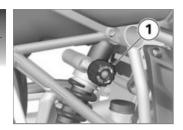
Your motorcycle's handling will suffer if you do not match the spring-preload and damping-characteristic settings. Adjust the damping characteristic to suit the spring preload.◀
