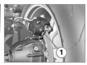
Visually inspect the brake pads to ascertain their thickness. Viewing direction: From the rear toward brake pads 1.
