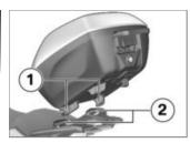
Hook the topcase into position on the luggage carrier. Make sure that hooks 1 are securely seated in the corresponding keepers 2.
