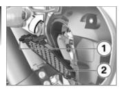
Hold the cover in position at the bottom on connector 2 and secure retaining hooks 1 at the top.
