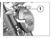
Swing the headlight back to its original position and install screw 1.
