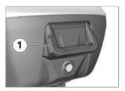
Pull handle 1 up as far as it will go.  Lift the topcase at the rear and remove it from the luggage carrier
