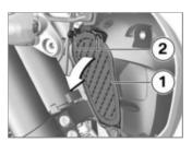
• Remove cover 1 by pulling retaining hooks 2.
