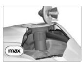
Refuel with fuel of the grade stated above; do not fill the tank past the bottom edge of the filler neck.
