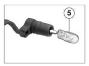
Press bulb 5 into the socket.
