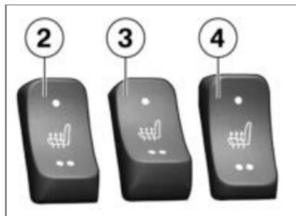
The rear seat has two-stage heating. Stage two is for heating the seat quickly: it is advisable to switch back to stage one as soon as the seat is warm.
