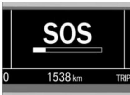
The time remaining until transmission of an emergency call is displayed on the progress bar. During this time, the emergency call can be cancelled by pressing and holding the SOS button.
