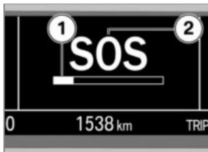
A progress bar **1** is displayed below the emergency call symbol **2** during connection setup.
