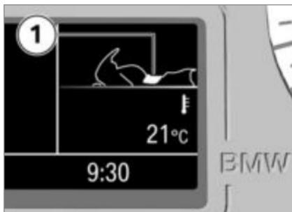
Symbol **1** appears on the display, indicating that the seat heating is ON.
