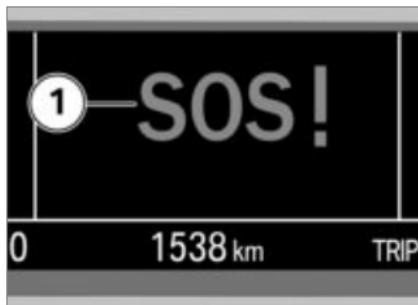
If emergency calls are not possible as a result of a technical fault, the symbol **1** is displayed.
