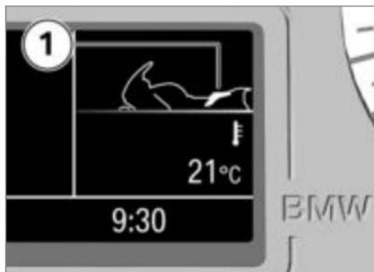
Symbol **1** appears on the display, indicating that the rear seat heating is ON.
