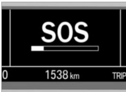
The time remaining until transmission of an emergency call is displayed on the progress bar. During this time, the emergency
