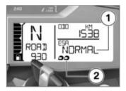
In the multifunction display, the damping is shown in area **1**, the spring preload in area **2**.
