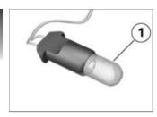
• Insert bulb 1 into the socket.
