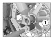
• Tighten right axle clamping screw 1 to the specified torque.
