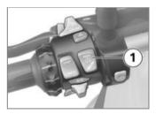
Press and hold button 1 until the ASC indicator and warning light changes its status.
