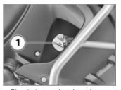
Check the coolant level in expansion tank 1.
