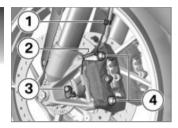
Install securing screws 4 on left and right and tighten to specified tightening torque.
