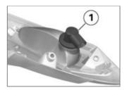
Insert bulb holder 1 into the bulb housing and turn the bulb holder clockwise to latch it in position.  Installing flashing turn indicator with fairing panel (m 119).
