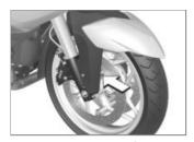
Visually inspect the left and right brake pads to ascertain their thickness. Viewing direction: Between wheel and front suspension toward the brake calipers.
