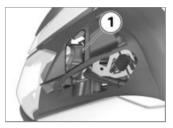
• Remove the side-light bulb through opening **1**.
