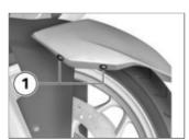
Remove screws 1 on left and right.  Work the front-wheel cover forward to remove, pulling the two sides slightly apart.
