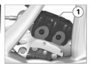
Visually inspect the brake pads to ascertain their thickness. Viewing direction: From the left toward brake caliper 1.
