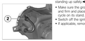
Insert the bulb holder into the headlight housing and turn lever 2 clockwise to latch it in position.
