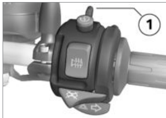
1 Emergency off switch (kill switch)
