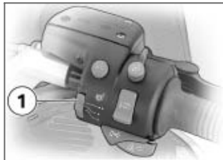
1 Switch for seat heating, front seat
