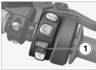
1 Emergency on/off switch (kill switch)
