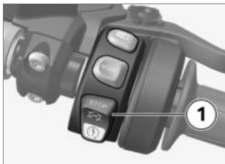
1 Emergency on/off switch (kill switch)
