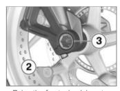
Raise the front wheel, insert quick-release axle 3 and tighten to specified torque. Quick-release axle in threaded bush (wheel carrier)
