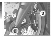
Once the calipers have been removed, there is a risk of the brake pads being pressed together to the extent that they cannot be slipped back over the brake disc on reassembly.
