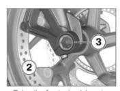
• Raise the front wheel, insert quick-release axle **3** and tighten to specified torque.
