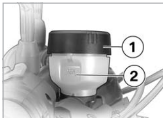
1 Front brake-fluid reservoir 2 MIN mark
