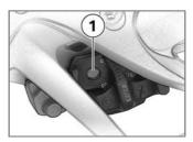
Brake-pad thickness, rear Make sure that the brake disc is not visible through the bore **1** in the inboard brake block.
