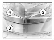
• Pull off the connector **3** beneath the headlight.
