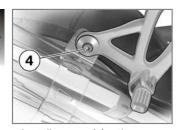
Install screw 4 for the bracket of the end silencer in the rear footrest, but do not tighten it at this point.
