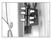
Brake-pad thickness, front The wear indicators on the brake pads must be clearly visible.
