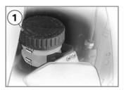
Check the brake fluid level in reservoir 1. The brake fluid level in the reservoir does not drop as the brake pads wear.
