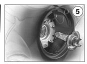
When installing, make sure that tab 5 is pointing up.
