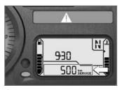
If the motorcycle covers long distances in the course of the year, under certain circumstances it might be necessary to have it serviced at a date in advance of the forecast due date. If the countdown distance to the odometer reading at which a service will be due is less than 1000 km, the distance is counted down in steps of 100 km and is shown briefly after the Pre-Ride Check completes.
