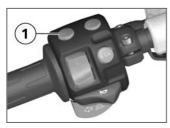
• Press and hold down button **1**. » Average speed is reset to zero.
