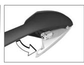
Pull the bulb housing out of the mirror housing at the threaded-fastener side.
