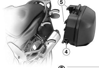
Warning: Always make sure that the cases are secured. An incorrectly secured case could be lost and endanger other road users.
