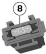
Fuse 8 for radiator fan
