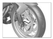
Visually inspect left and right brake pads from the front to determine their thickness. Direction of view: between wheel and front suspension to brake calipers.
