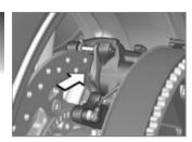
Check the brake pad thickness with visual inspection. Direction of view: from rear at brake caliper.
