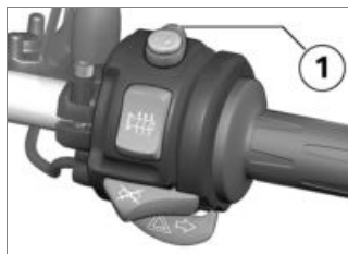
1 Emergency-off switch (kill switch)
