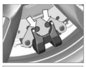
Brake-pad wear limit of parking brake
