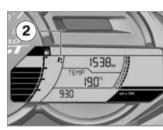
The set level 2 is shown in the display. The second stage is used to quickly heat up the passenger seat; then the switch should be switched back to the first stage. The following displays are available:
